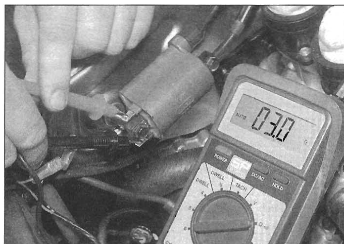
3.4 Checking the coil primary circuit resistance
