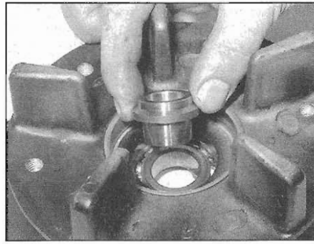
16.25a Remove the spacer . . .
