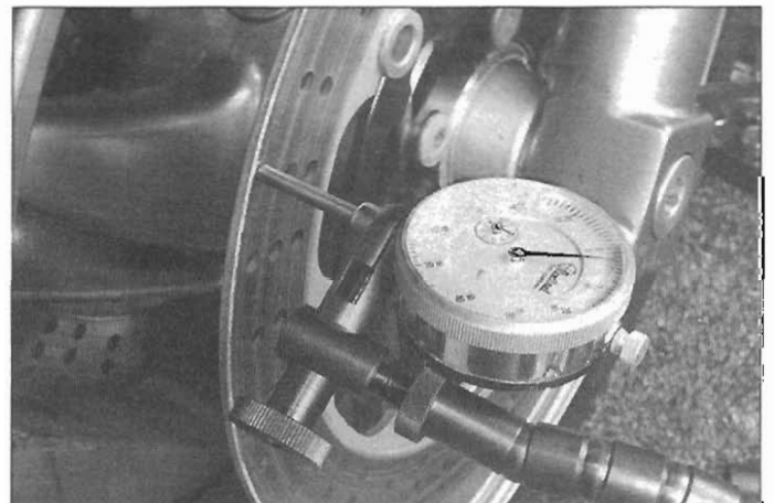
4.2 Set up a dial gauge, with the probe touching the disc, and turn the wheel to measure runout
