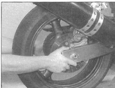
22.8a Checking for play in the swingarm bearings
