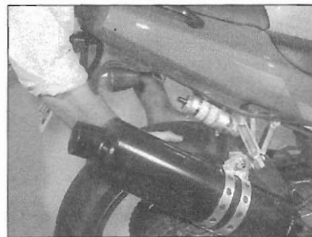
22.8b Checking for play in the suspension and linkage
