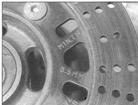
8.3 The minimum thickness is stamped into the disc
