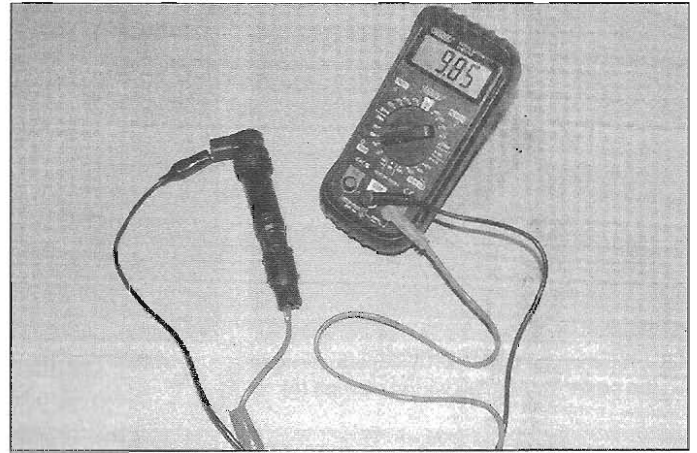
3.14 Measuring the coil/cap secondary resistance
