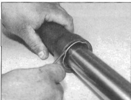
7.11 Pry out the retaining clip using a flat-bladed screwdriver
