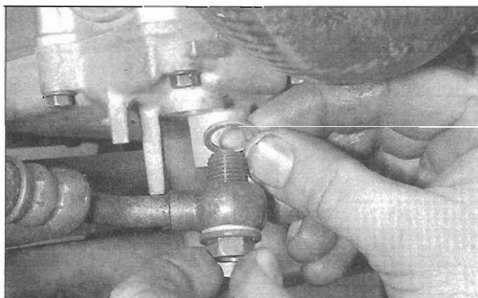
10.8 Fit a new sealing washer on each side of the unions
