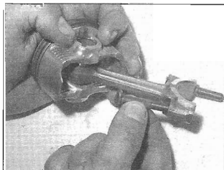
27.24a Fit the new bolts into the rod
