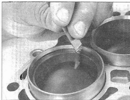
15.3 Measuring piston ring installed end gap
