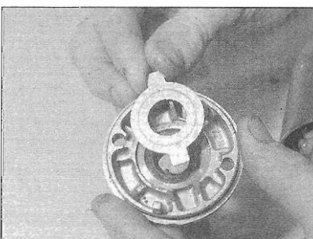
29.32 Fit the tabbed washer into the front cover
