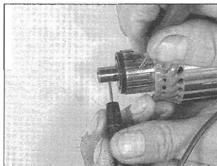
29.18b There should be no continuity between the commutator and the armature shaft
