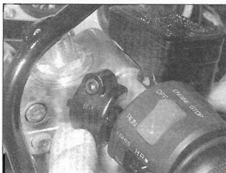
5.3b Unscrew the clamp bolts and detach the master cylinder assembly
