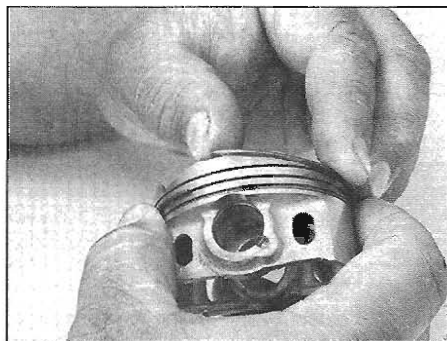
15.7 Fit the second (middle) ring into the middle groove in the piston
