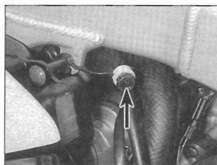
13.3b Idle speed adjuster (arrowed) – G, H, J and A models
