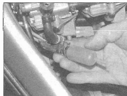
20.11 Detach the heater filter from the coolant hoses
