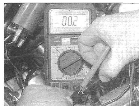
31.12 Checking stator coil resistance
