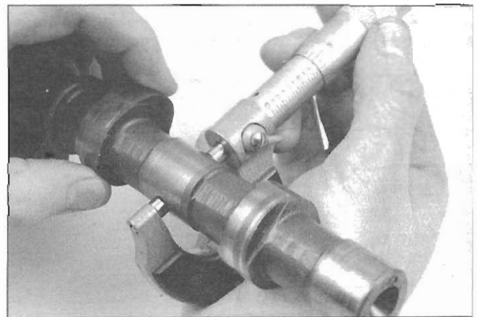
9.15b Measure the cam bearing journals with a micrometer
