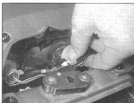
9.2 Remove the bulbholder from the tail light . . .
