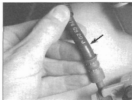
10.3 Flex the brake hoses and check for cracks, bulges and leaking fluid
