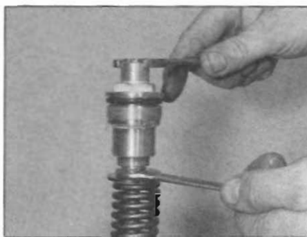
7.5 Counter-hold the locknut and unscrew the top bolt assembly using a spanner on the flats of the pre-load adjuster
