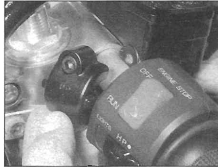
5.23 Install the clamp with the UP mark facing up
