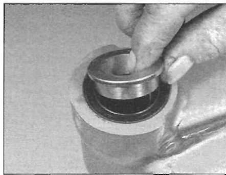
14.4a Remove the collar and cap . . .
