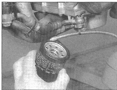
19.7a Smear oil onto the sealing ring ...
