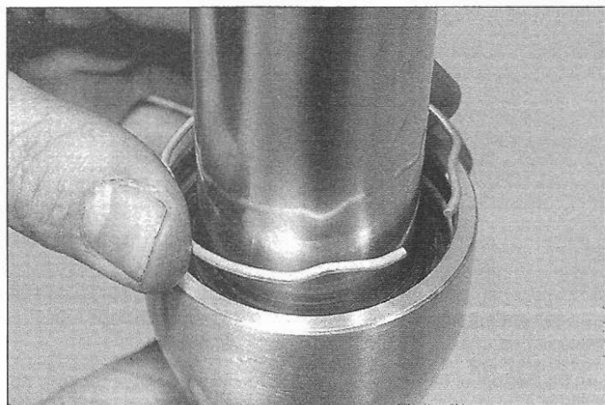
7.24 Install the retaining clip ...
