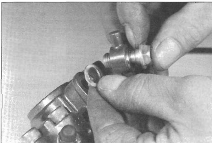
3.17 Always use new sealing washers on each side of the hose union
