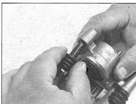
7.10b Check the condition of the rubber boots and replace them if necessary
