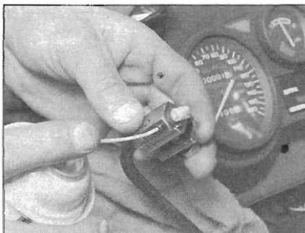
15.3a Lubricating a cable with a pressure lubricator. Make sure the tool seals around the inner cable
