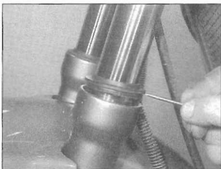
22.3 Checking for leakage of the fork seals
