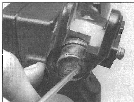
5.11 Remove the rubber boot from the end of the master cylinder piston . . .
