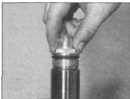
7.4 Unscrew the top bolt from the fork tube
