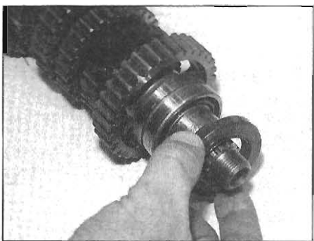
29.5 Replace the output shaft oil seal if required
