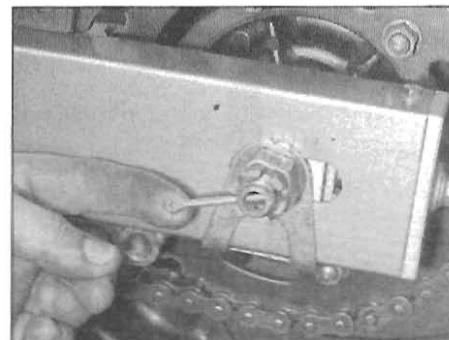
2.8b ... then secure it using a new split pin
