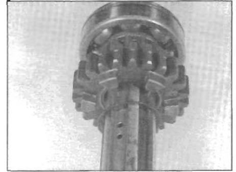
31.7b ... the toothed washer and 5th gear ...
