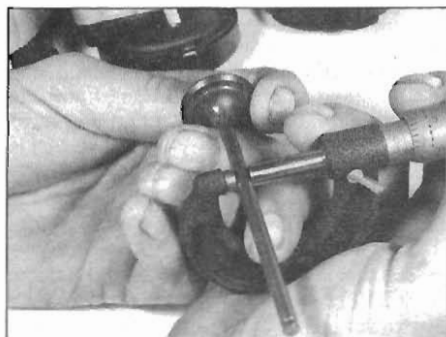
12.17a Measure the valve stem diameter with a micrometer
