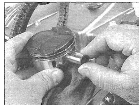
14.4b . . . then push the pin out and withdraw it from the other side of the piston
