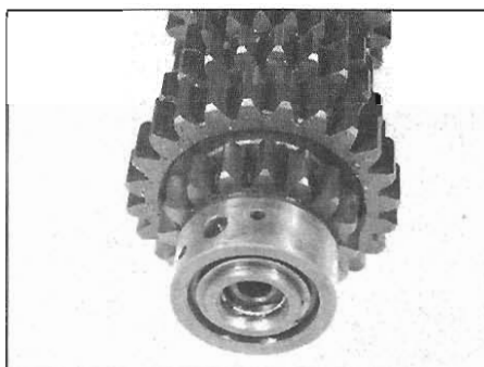
31.2a Slide off the needle bearing outer race . . .
