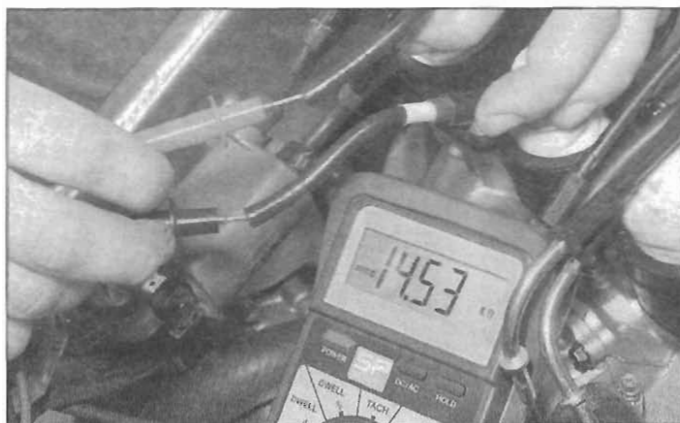
3.6 Checking the coil secondary circuit resistance
