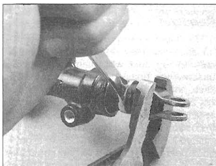
9.7b Hold the clevis and slacken the locknut
