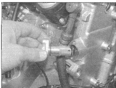
8.10b ... then install the tensioner ...
