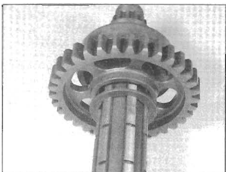
31.19b ... the toothed washer and 2nd gear ...
