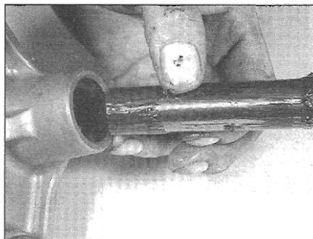
11.14 Coat the spacers with moly-grease before installing them
