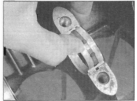
26.4 To remove a main bearing insert, push it sideways and lift it out
